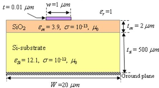
**Figure 1 Cross-section of single interconnects line on Si-SiO<sub>2</sub> substrate.**
