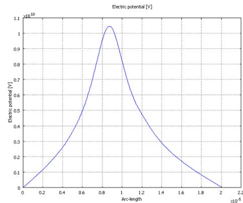
**Figure 8 Potential distribution of coupled interconnects line on silicon-silicon oxide substrate from  $(x,y) = (0,500 \mu\text{m})$  to  $(x,y) = (20 \mu\text{m}, 502 \mu\text{m})$ .**
