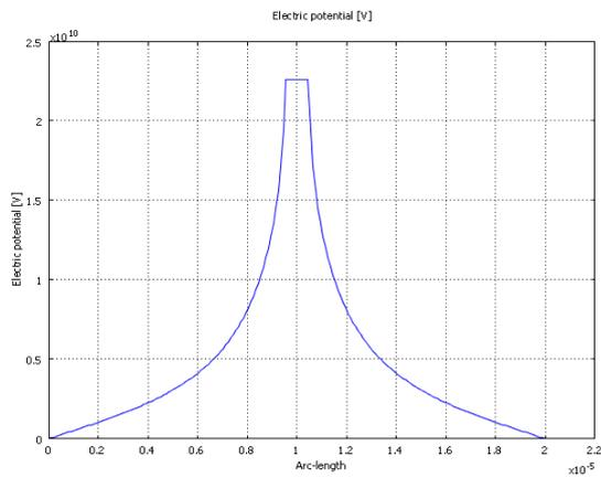
Figure 2 Potential distribution of single interconnect line on Si-SiO<sub>2</sub> substrate from (x,y) = (0,502 μm) to (x,y) = (20 μm, 502 μm).
