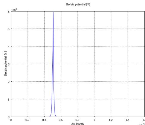
**Figure 9 Potential distribution of coupled interconnect lines on silicon-silicon oxide substrate from  $(x,y) = (0,0)$  to  $(x,y) = (20 \mu\text{m}, 1500 \mu\text{m})$ .**
