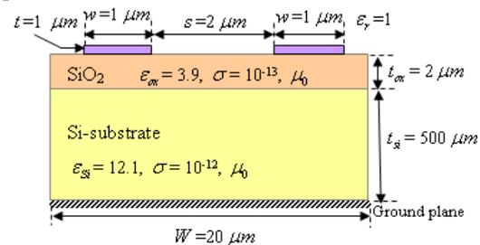
Figure 6 Cross-section of coupled interconnect lines on Si-SiO<sub>2</sub> substrate.
