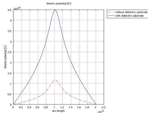
Figure 5 Comparison analysis of potential distribution of single interconnects line on Si-SiO<sub>2</sub> substrate from (x,y) = (0, 500 μm) to (x,y) = (20 μm, 502 μm).
