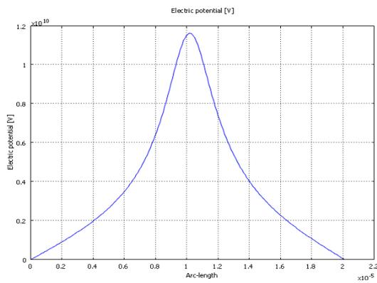
Figure 3 Potential distribution of single interconnect line on Si-SiO<sub>2</sub> de substrate from (x,y) = (0,500 μm) to (x,y) = (20 μm, 502 μm).
