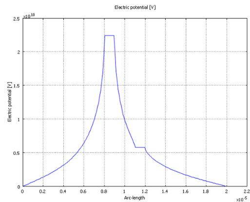
**Figure 7 Potential distribution of coupled interconnect lines on silicon-silicon oxide substrate from  $(x,y) = (0,502 \mu\text{m})$  to  $(x,y) = (20 \mu\text{m}, 502 \mu\text{m})$ .**
