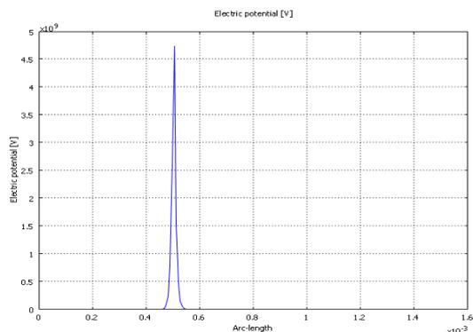
Figure 4 Potential distribution of single interconnect line on Si-SiO<sub>2</sub> substrate from (x,y) = (0,0) to (x,y) = (20 μm, 1500 μm).
